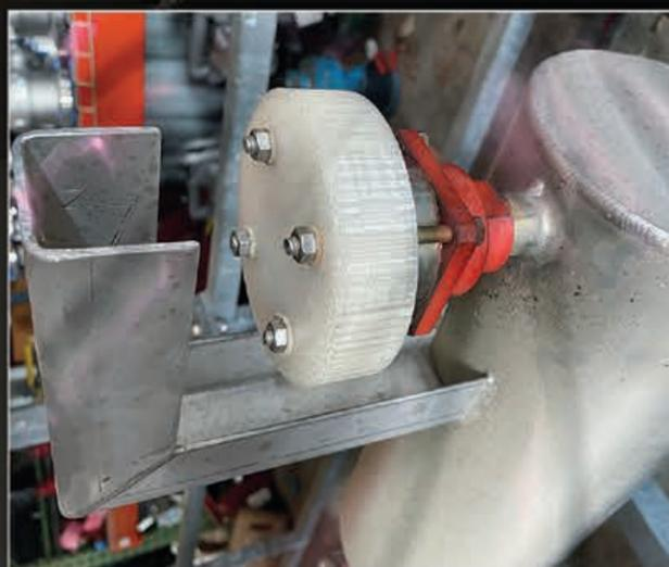
“The unique part about the flame arrestor cap is that the part used in the High Lift is the same as the one in the Pantograph systems that we use for Hot-Pit refueling,” said SrA Sasser. “In the event there is an issue with a pantograph cap, we now have the means to return them to service quickly.”
